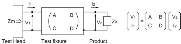
2. The impedance of chip coil  $Z_x$  and measured value  $Z_m$  can be described by input/output current/voltage.
