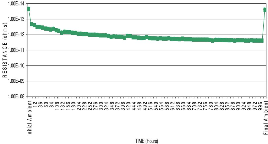
Surface Insulation Resistance:  $> 1 \times 10^{11} \Omega$ , passed.
