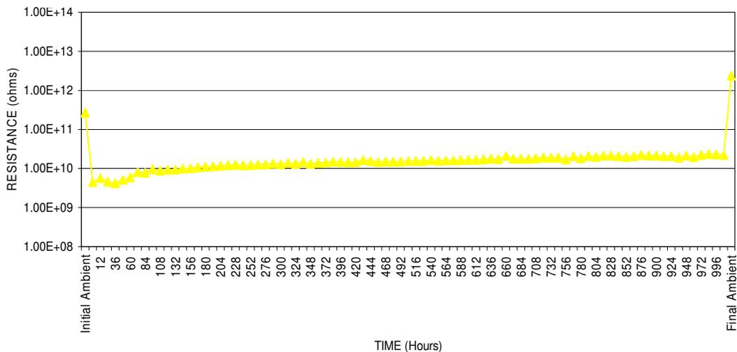
Surface Insulation Resistance: > 1 x10<sup>9</sup> Ω, passed.
