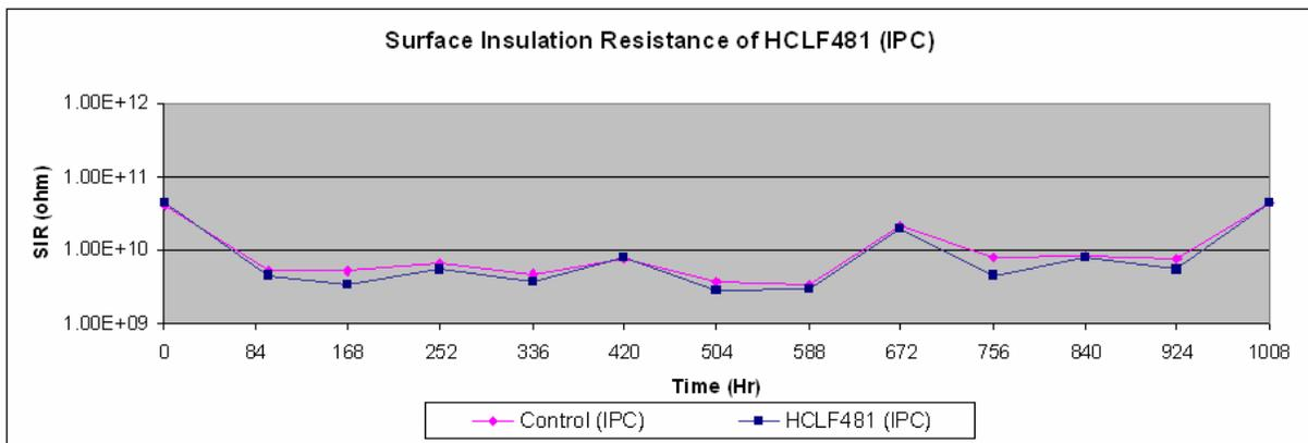
Surface Insulation Resistance:  $>1 \times 10^9 \Omega$ , Pass.
