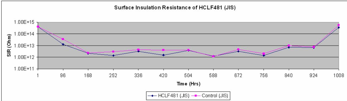
Surface Insulation Resistance:  $>1 \times 10^{12} \Omega$ , Pass.
